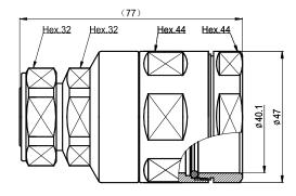
7/16 Straight male Connector for 1-1/4 Flexible RF Cable
