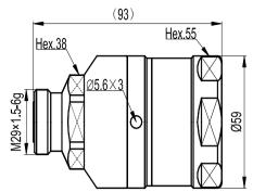
7/16 Straight Female Connector for 1-5/8" Leaky Cable
