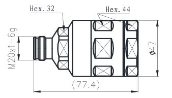
4310 Straight female Connector for 1-1/4 Flexible RF Cable
